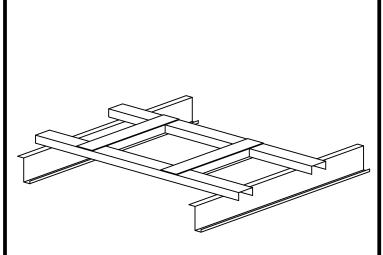
Place side supports on purlins. Attach upper and lower end supports to side support. Do not attach side supports to building structure.
